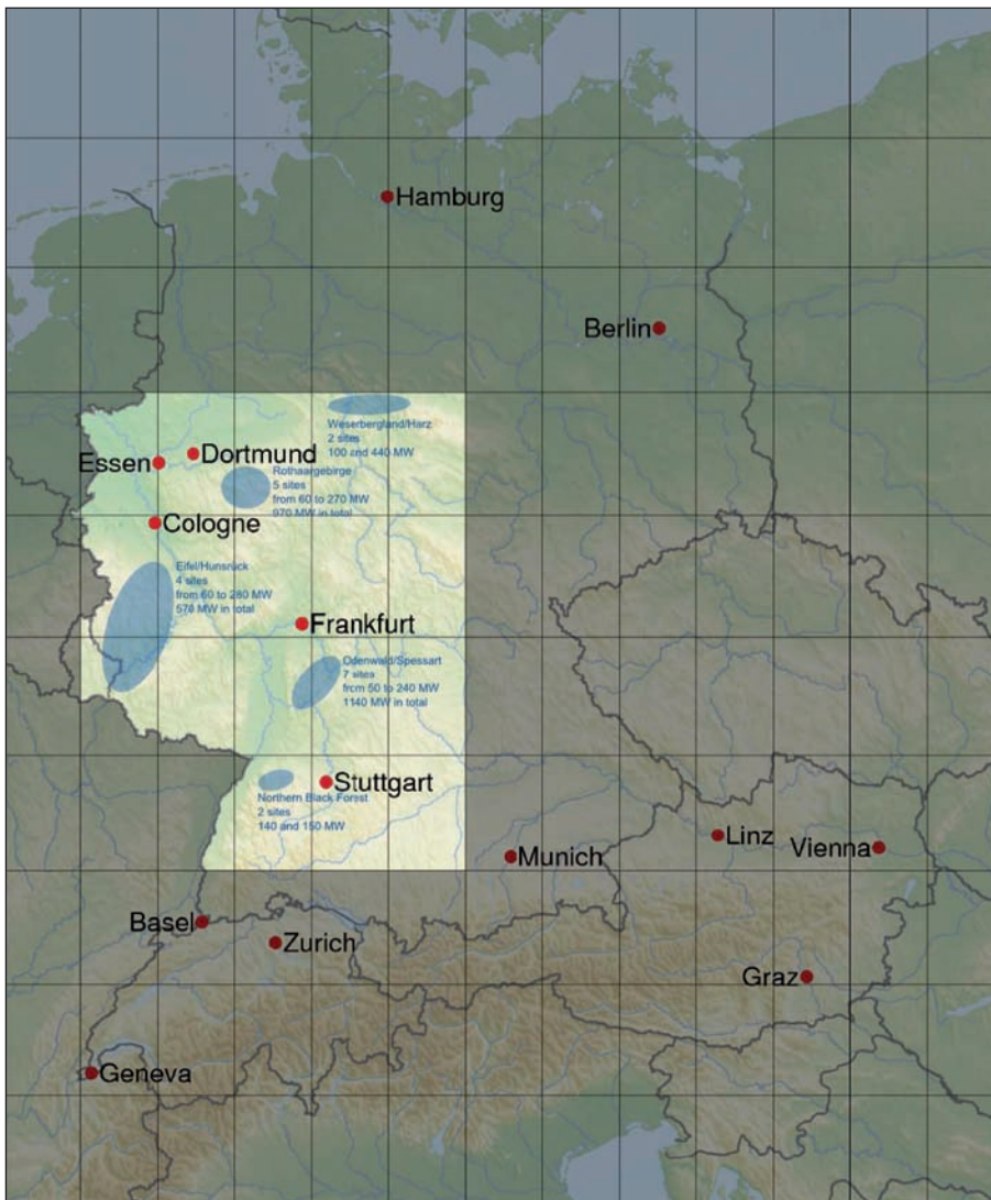
Figure 6. Result of a systematic study of PSP potential between 48° and 52° latitude and 6° to 11° longitude, respectively (RWE internal).
